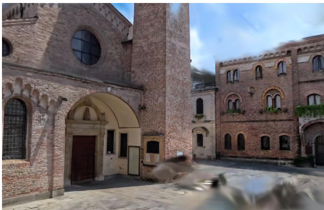
Figure 1 – The Piazzetta di San Nicolò in Padua reproduced with the gaussian splatting survey method using PostShot software
