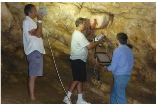
Fig. 5: pXRF study of the pigments of painted figures at the Genovesse cave
