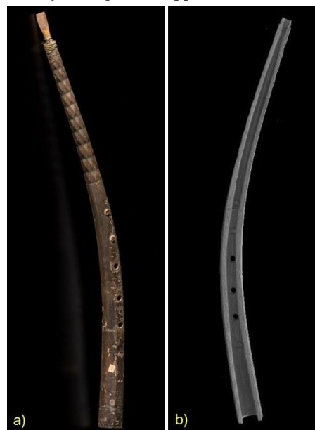
Figure 1- CT scan of a woodwind musical instrument. (a) Picture of the cornetto (L=580 mm; D= 7.5÷26.5 mm). (b) 3D rendering of the whole object. Virtual cut along the vertical direction.
