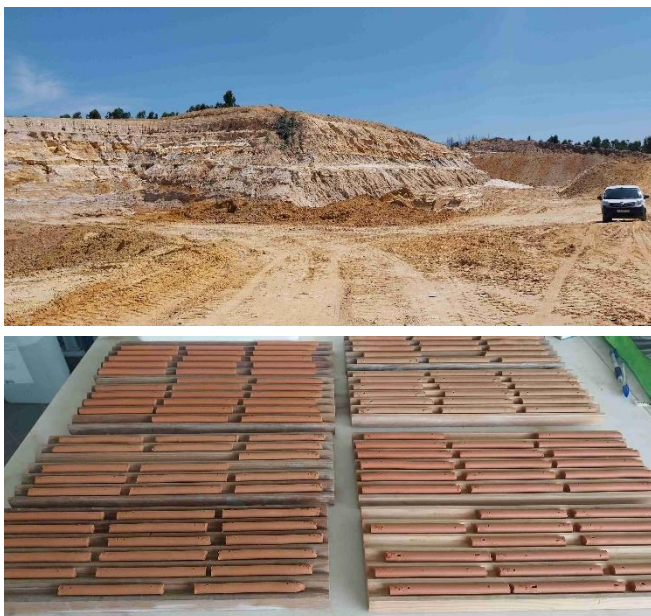
Figure 1 - Current clay quarries in Vale Coimbra area (above) and some of the testing probes prepared for the flexural strength determination (below).
