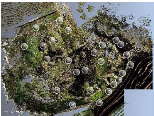
Fig. 3. 3D point cloud with indication of the 3D scanning stations.
