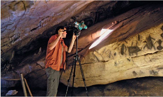
Fig. 4: Genovesse cave, light structured 3D scanning mapping (Tusa et alii 2013).
