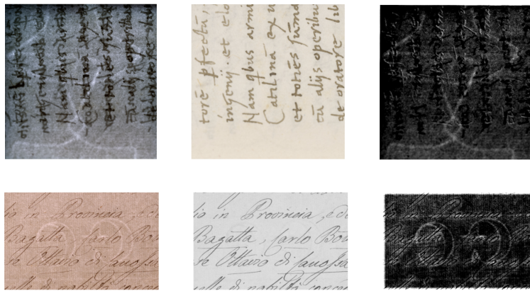
Figure 2: Transmission-mode image T , reflection-mode image (front side) R , and the watermark W signal. (top) 15th century, code CCLVII (229). (bottom) notarial deed (1864).
