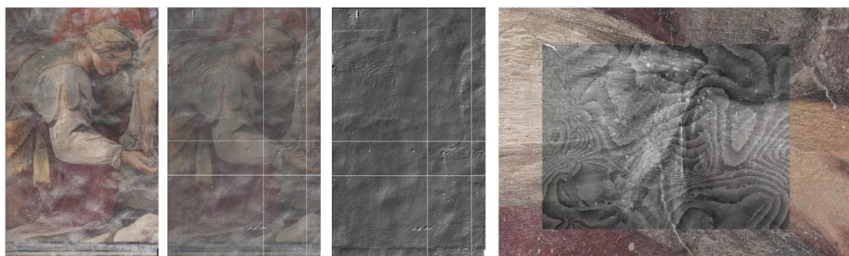
Figure 1 – TLS and Digital Photogrammetry 3D reconstruction of the wall painting representing “the Deposition of Christ” counter façade: comparison between DHSPI and DP ortophoto on a detail of the artwork.
