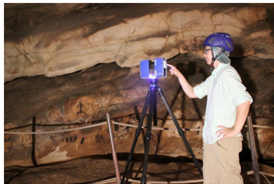
Fig. 3: Genovese cave, terrestrial laserscanning (TLS) mapping
