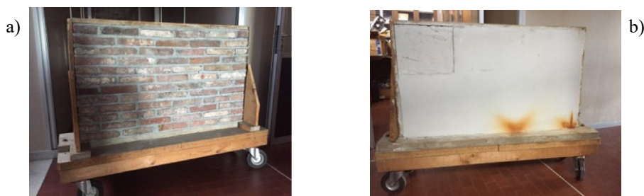
Figure 1 – Back side (a) and front side (b) of the mock-up of masonry wall used for measurement
